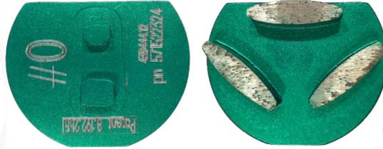
The 3SEG Oval Tool is a metal bond preparation tool that has the EG attachment system as a standard for use on any Prep/Master Machines. Its uses are to remove adhesives, thin-sets, surface inequalities of +/-4mm and epoxy coatings with thickness of
